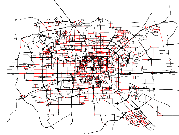
Figure 15: A map of Beijing, with a spanning tree shown in black, and the remaining loop-closing constraints shown in red. A spanning tree can be used as a preconditioner by GTSAM.
